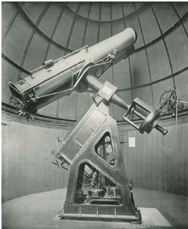
Figure 5. The Grubb astrographic refractor at Greenwich Observatory.
